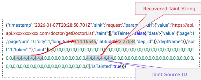
Fig. 7: An example of byte-level taint recovery at a network sink. MINNIE recovers the concrete payload fields carrying sensitive data (e.g., longitude and latitude) and associates them with their corresponding taint source identifiers, providing direct runtime evidence of privacy leakage.
